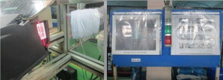
BAR CODE SCANNING SYSTEM IN COWL TOP ASSY FOR SPEC ERROR
