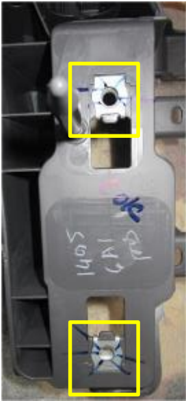
POKA – YOKE FOR SPRING NUT MISSING
