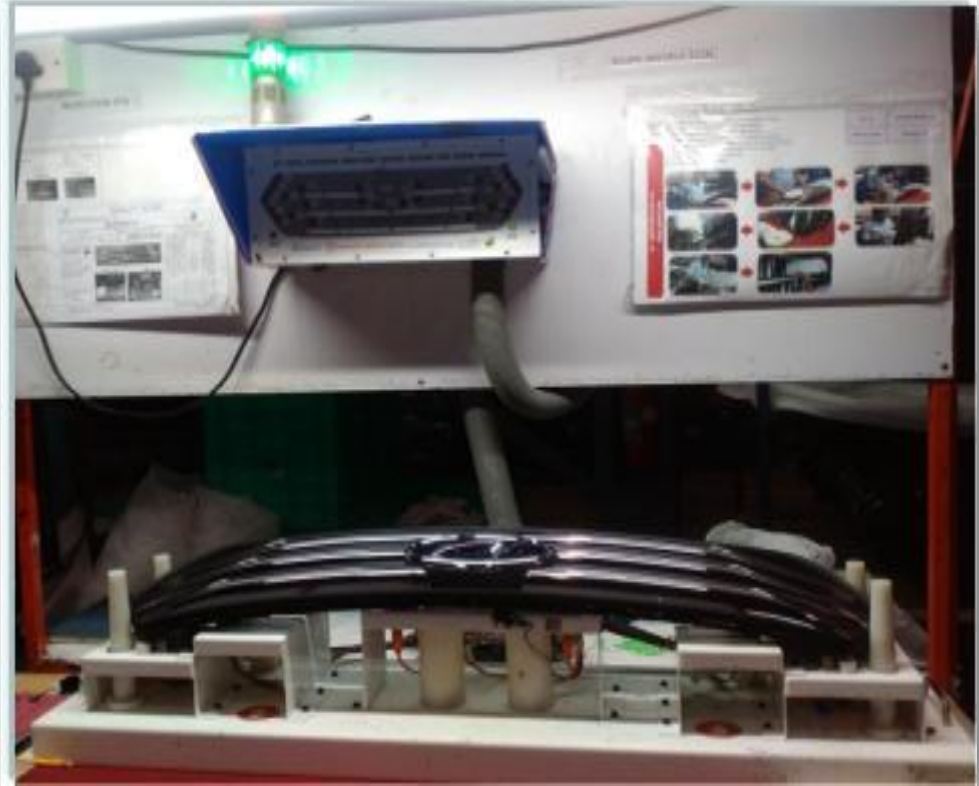
GRILLE RADIATOR ASSY SCREW MISSING POKA YOKE SYSTEM (28 No's)
